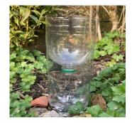
Find an open place outside for your bottle. it Dig it slightly into the ground and weigh it down with stones. Remember to record how much rain falls with your rain gauge
