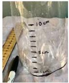
Using your pen and ruler, mark a vertical scale on the bottle. We have marked every cm. Pour the water back in. Turn the top upside down and put in the base as a funnel
