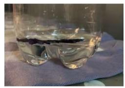
Pour the 100ml water into the bottle base and mark this level with your pen. Empty the water back into the container for now. This line is where you will start your scale from
